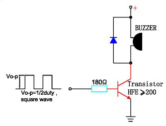
The base current Ib should high enough so that it saturates the collector current of the transistor with the CB load.
